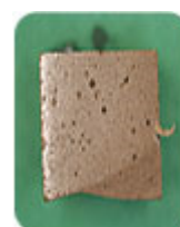
Photo 2: This image depicts epoxy #3 after two weeks of daily applications of used cooking oil and a properly diluted enzymatic cleaner. The surface has softened (note the easily made scrape on right) and is more porous than the epoxy depicted in Photo 1.
