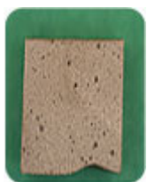
Photo 1: This photo depicts the surface of the control sample of epoxy #3 (no exposure).
